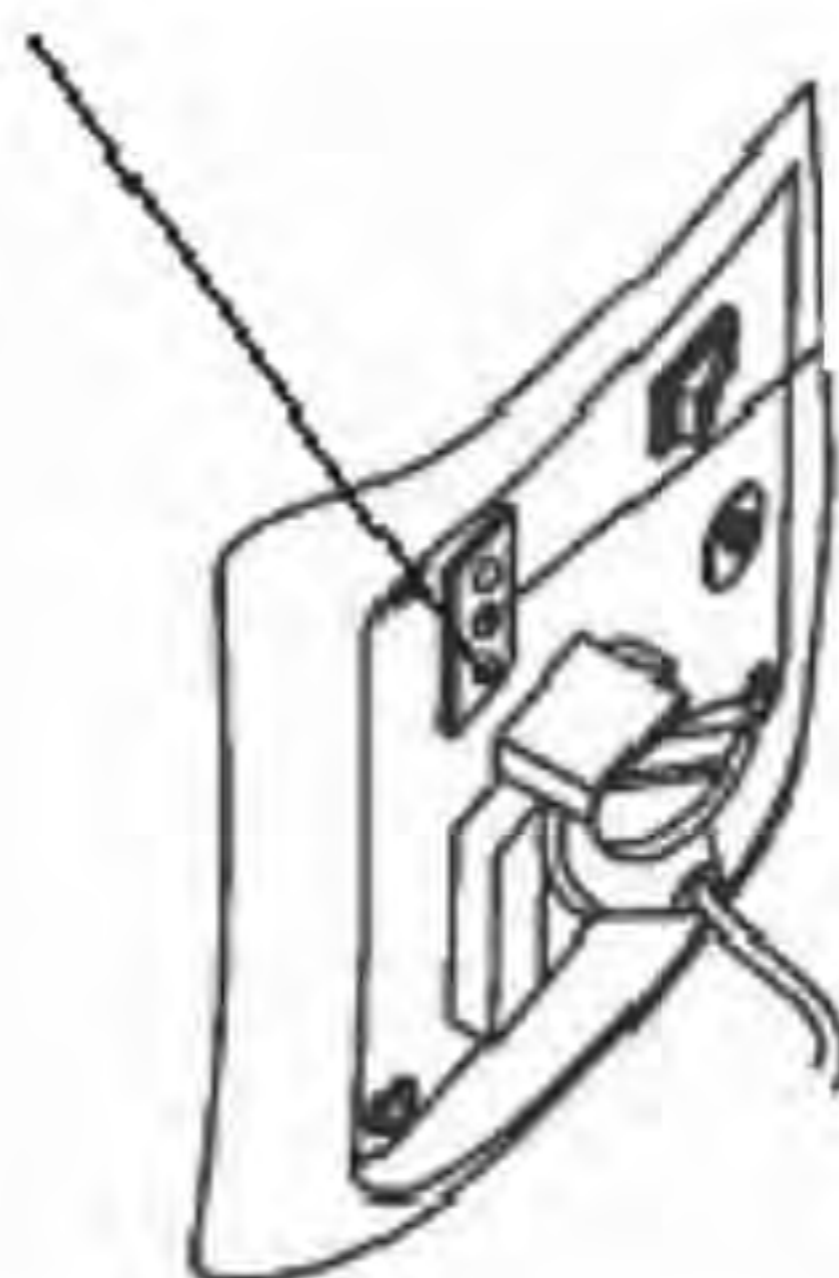
Low oil alarm Indicator Light (Red)
