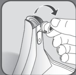
**EN** Remove the water inlet stopper.
