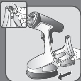
**EN** Return the water tank to its place on the appliance. Make sure the water tank is fully set in place and locked.
