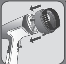
The fabric brush opens the weaves of the fabrics for better steam penetration. Before removing or attaching the steam brush, unplug your appliance and allow it to cool down, for one hour.
